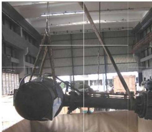
Fig.19. Handling a welded end valve with an extended stem
