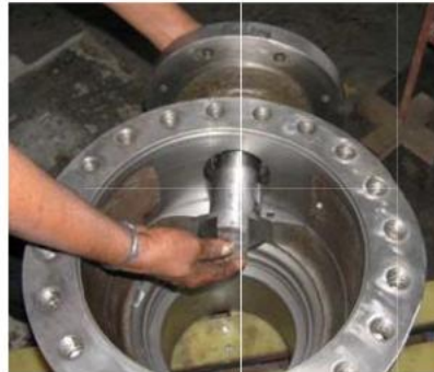
Fig.10. Stem being inserted into the body
