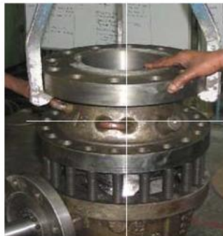
Fig.14. Connector being placed on the body.
