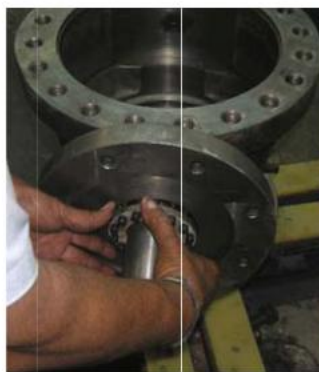
Fig.11. Gland packing inserted into the body
