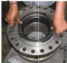
Fig.13. Seat ring being inserted into the connector
