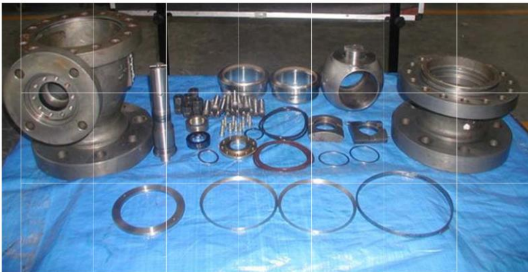
Fig.8. Major components of valve before assembly
